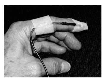
Figure 5. Thermistor placement at the fingertip.
