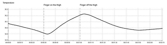
Figure 6. Thermistor warming due to contact with the thigh.
