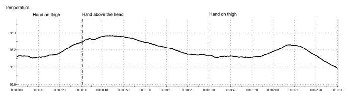
Figure 8. Effect of hand position with respect to the heart on skin temperature.
