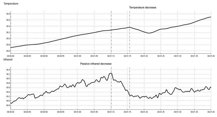
Figure 3. Comparison of thermistor and passive infrared (pIR) signals.
