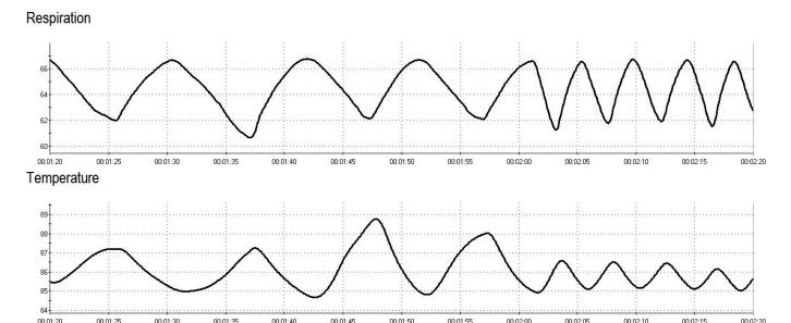
Figure 10. Respirometer and nasal thermistor waveforms.
