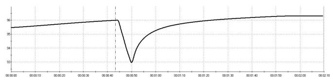
Figure 7. Thermistor decoupling due to movement.
